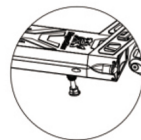
Fasten the glue plug after charging
