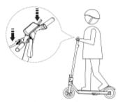
To slow or stop the scooter, release trigger and hold the handbrake.
